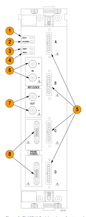
Figure 2: TLA7S16 Serial analyzer front panel
