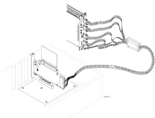
Figure 6: Connecting a slot interposer probe
