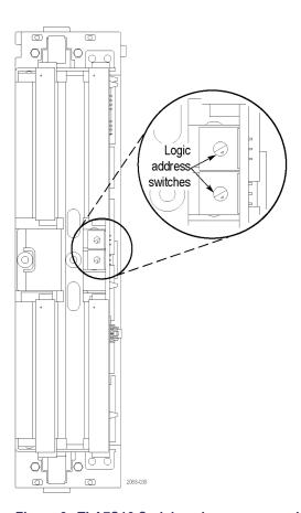
Figure 3: TLA7S16 Serial analyzer rear panel
