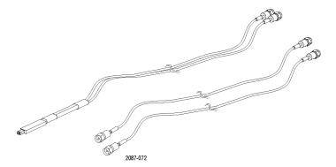
Figure 8: Clock cable and clock jumper cable
