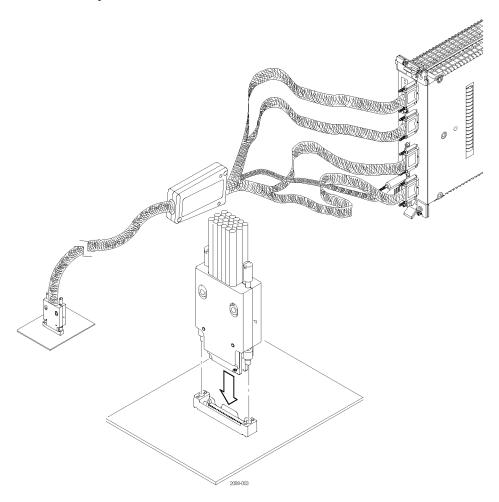
Figure 5: Connecting a mid-bus probe to your SUT
