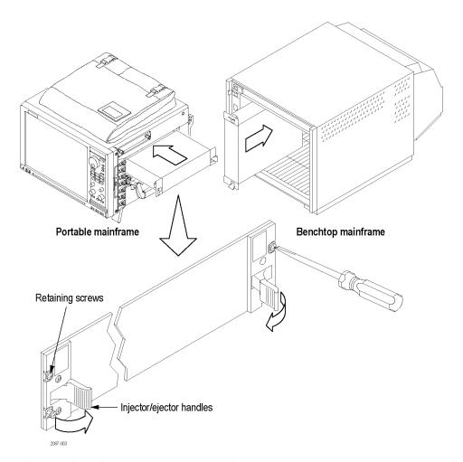
Figure 4: Installing a serial analyzer module
